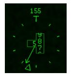
set to 155 knots). The Airspeed round dial has 10 tick marks surrounding the digital readout and the triangle on the outside points to the Selected Airspeed. The arrow pointer points to the current speed and the movement of the arrow pointer gives the pilot a sense of the speed trend.
