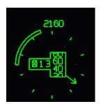
Altitude is shown above the round dial. The Vertical Speed worm around the Altitude round dial grows from the middle of the left side and indicates a positive vertical speed (climb) as the worm grows up from the middle of the dial and negative vertical speed (descent) as it grows down from the middle. The scale for the growth of the vertical speed worm changes as the vertical speed increases so that it is most sensitive for lower vertical speeds and less sensitive for higher vertical speeds.
