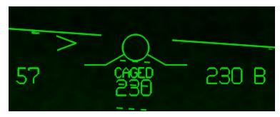
caret. When the aircraft is not accelerating or decelerating it is exactly to the left of the left wing tip. When the aircraft is accelerating, it moves above the left wing tip in proportion to the acceleration. Pilots can use the acceleration caret in conjunction with the speed readout. If they see that
